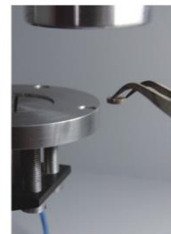
2 使用镊子将菌物载片转移到载物台上 Transferring the metal plate to objective table
